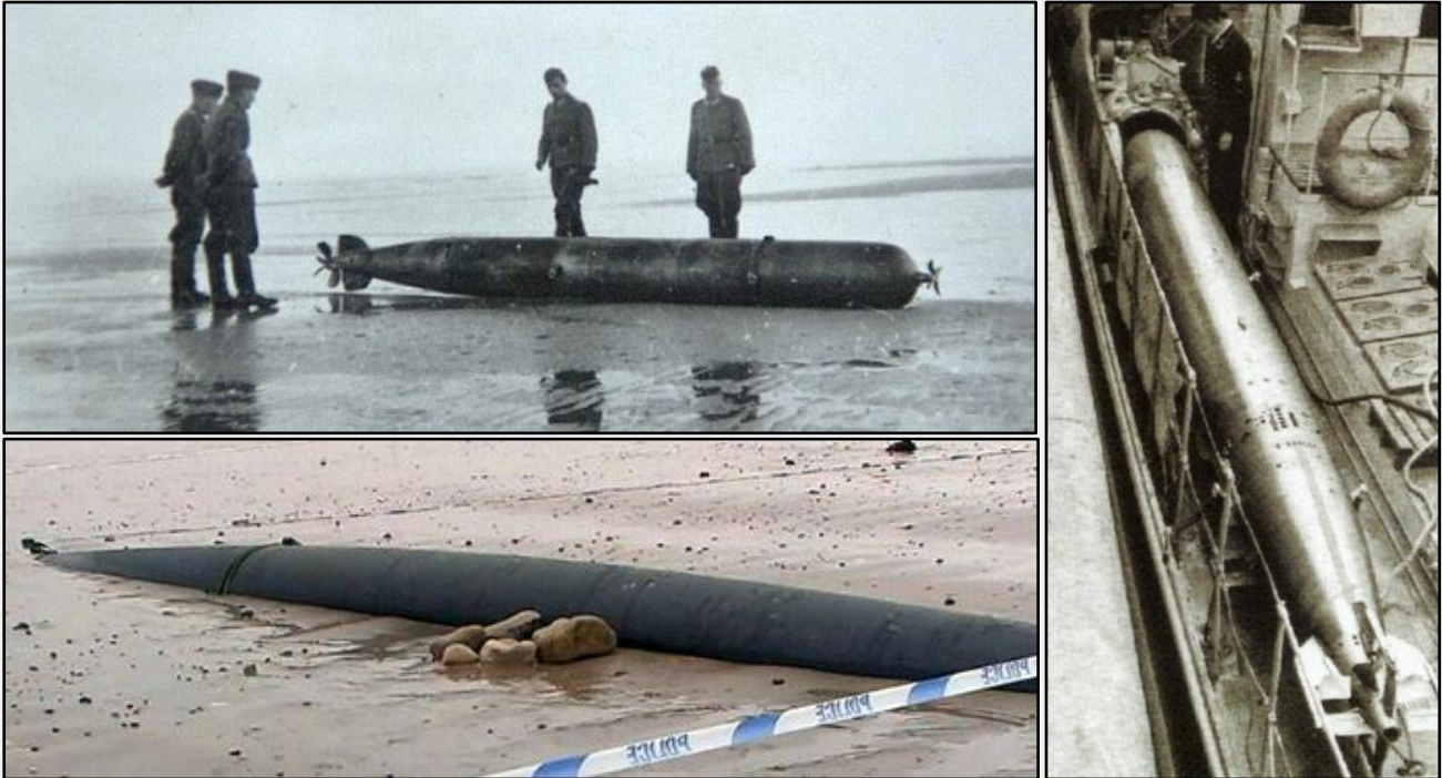
Typical examples of heavyweight (21in/53cm) torpedoes
