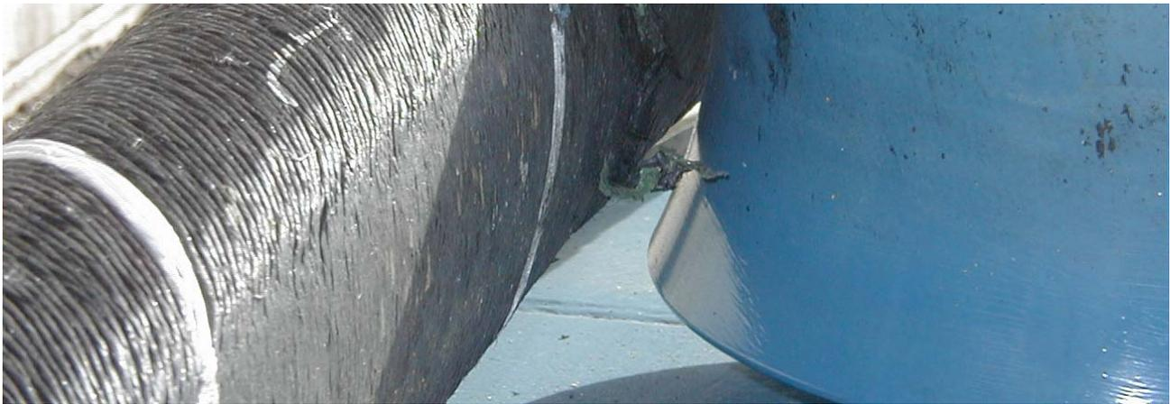
Figure 6-7. Example of destructive test in which a 3-core cable is moving against rollers which are too far away from each other. In the picture the rollers apply a sidewall force to the cable which is too high.
