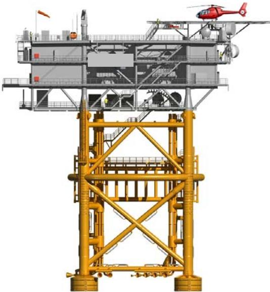
Figure 3-4. Illustration of a transformer platform with J-tube connections for submarine cables.
