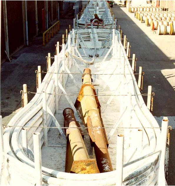
Figure 3-1. Coiling of cables on a train set.
