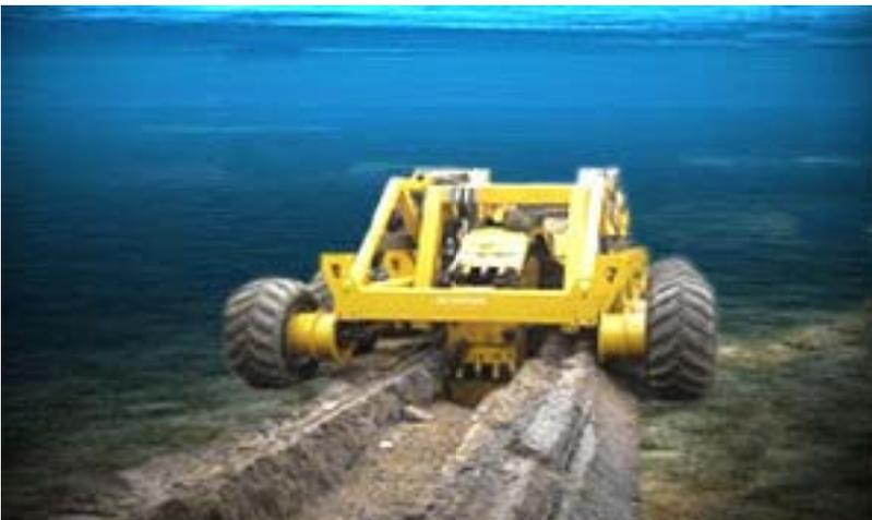
Figure 3-11. Example of a wheel trencher.
