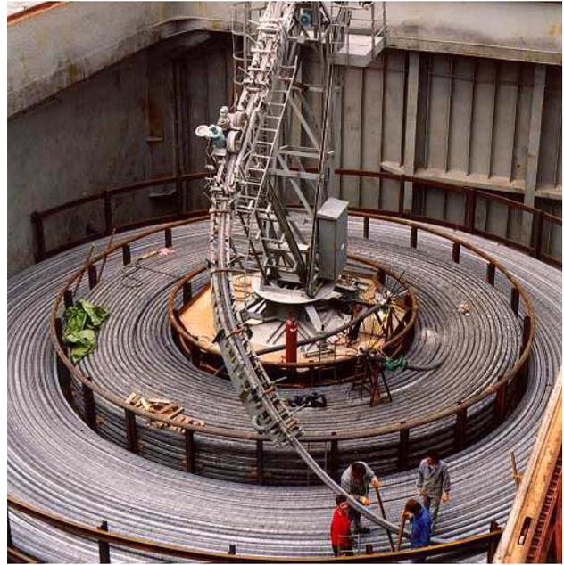
Figure 3-2. Storing cable on a turntable placed on a vessel.
