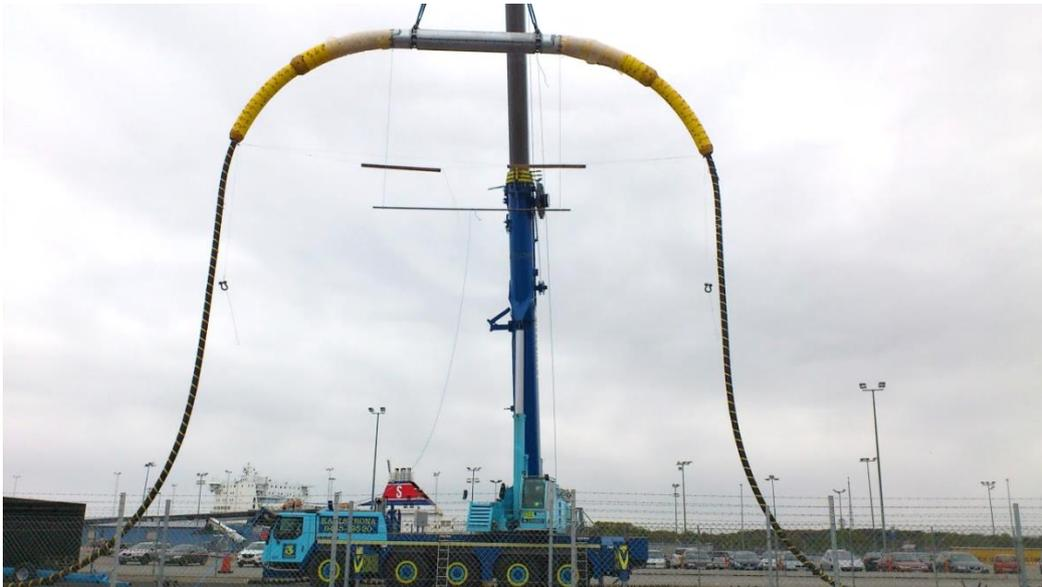
Figure 6-11. Example of handling test on rigid joint with bend restrictors.
