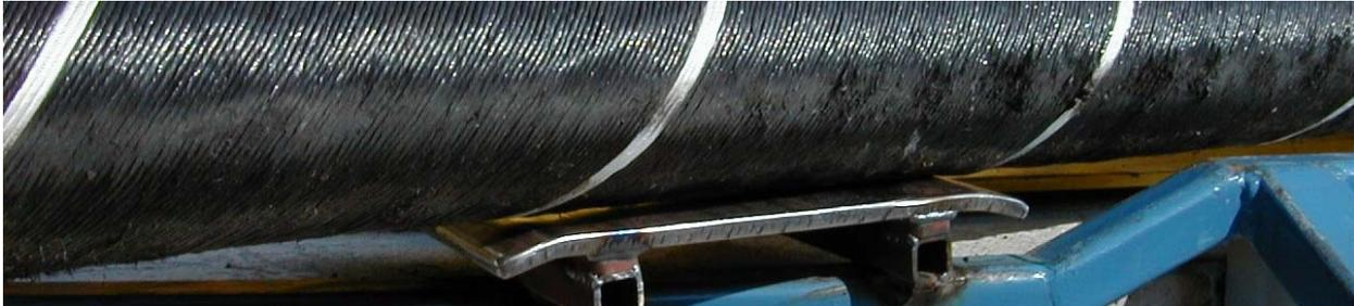
Figure 6-6. Example of simulation of cable moving against a guiding plate of a capstan wheel.
