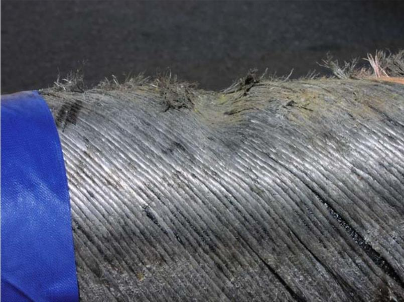
Figure 6-10. Photo of three core armoured cable after impact test.
